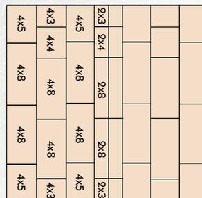
Above right: Layout pattern for 24' x 24' garage. 23 4'x8' panels are required.
