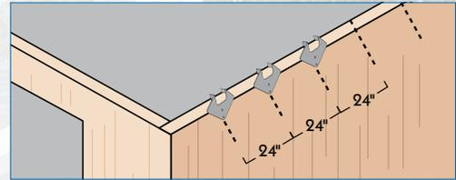
Just as you measured for spacing of the wall studs, you should begin by measuring and marking the locations for the roof trusses. (Pre-built roof trusses are specially designed to carry the load of the roof to the outside walls while saving considerable time during installation.)
