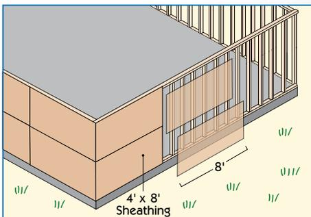
with the end of the wall and the bottom plate. For secure nailing, make sure that the edge of every panel falls on the middle of a stud and that it butts tightly with the next board.
