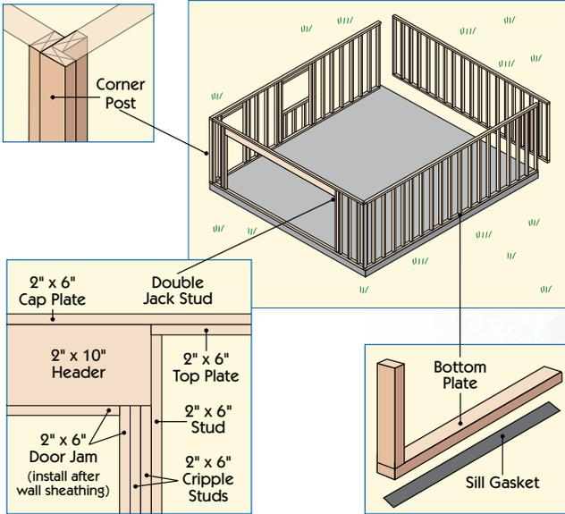
Before lifting the walls into place, construct the four corner posts as a unit and treat them as separate studs.
